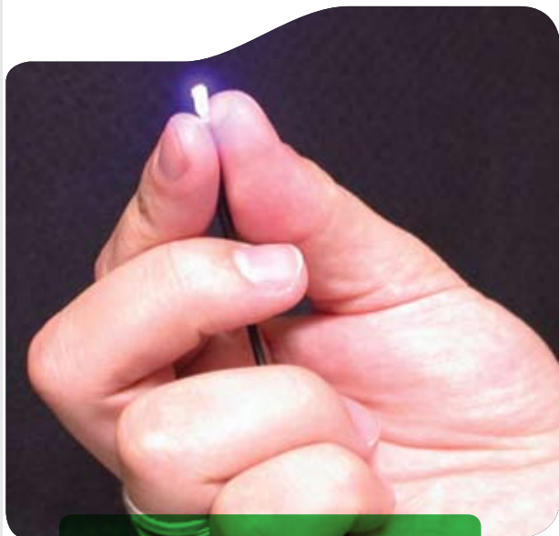
AN OPTICAL FIBRE WITH THE PORTABLE DOSIMETER MATERIAL ATTACHED TO THE END.
